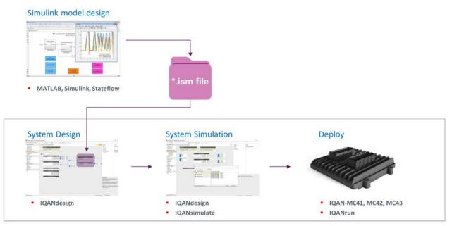
**Picture:** An .ism file is generated that is imported to IQANdesign, inport and outport can easily be connected to channels in the IQAN project file.
